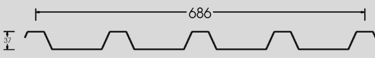
Type: IBR Sheet Profile : Standard IBR Section. Coil : 925mm wide, mild steel capacity 450 MPa UTS Thickness : 0.4 - 0.6mm. Coverage : ± 686mm.
